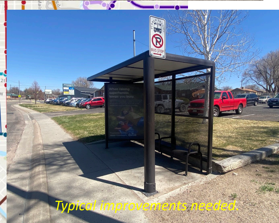
Existing bus stops are not ADA accessible and leave passengers vulnerable to weather conditions.
